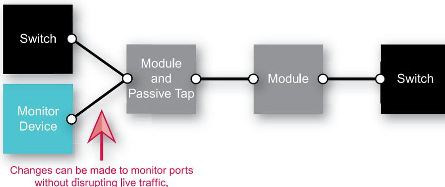
As you can see, this structured cabling solution for passive tapping also eliminates two connections (one jumper) from the link, which some network designers will find useful for their optical budgets at more extended distances.
