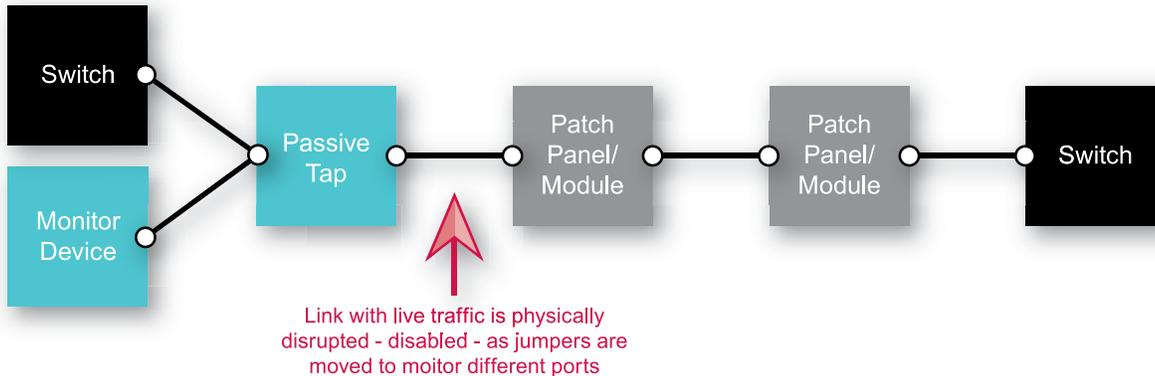
With Corning's Pretium EDGE Tap Module, the module serves as both the "patch panel" and the passive tap device. You can change the ports that are monitored without ever disrupting the flow of live traffic..
