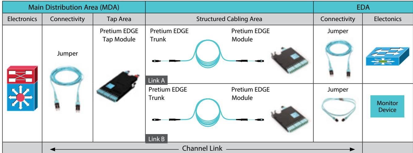
The advantage of this option is that it allows the monitoring electronics to be completely separated from the live network electronics, limiting network access to network administrators and monitoring access to data security/compliance administrators. However, this design is practical only for 10G Ethernet networks, as 8G Fibre Channel is limited to 5 metres in the monitor link.
